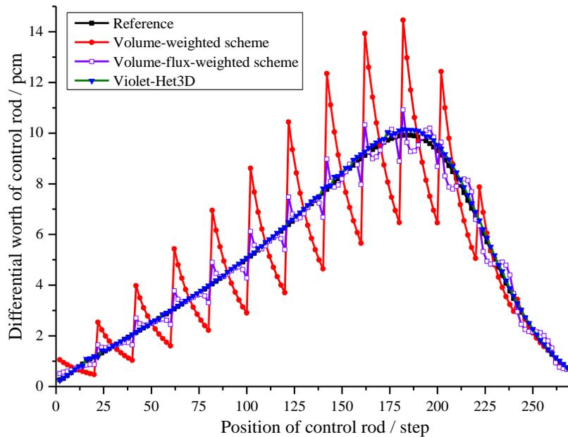
Fig. 8 Differential worth of control rod calculated by different scheme
