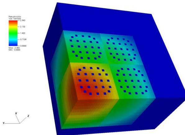
Fig. 3. Power distribution of the pin-by-pin problem
