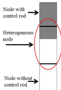
Fig. 7 Heterogeneous node caused by control rod
