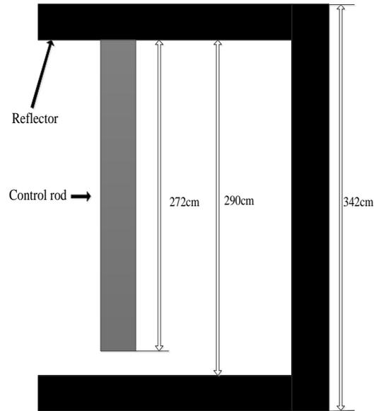
Fig. 6 Axial size of the reactor core
