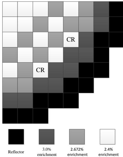
Fig. 5 Radial configuration of 1/4 reactor core
